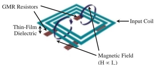
Figure 2: Magnetic coupler construction.
