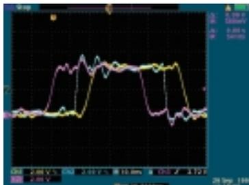
Figure 3: Magnetic couplers (blue trace) have faster rise, fall, and propagation times than the fastest opto-couplers (yellow trace) for the same input (purple trace).
