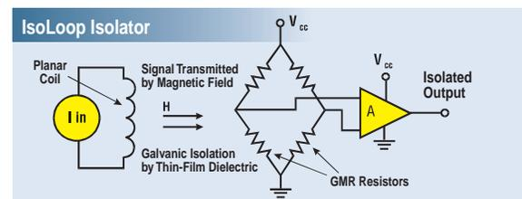
Figures 1a and 1b: Optical couplers compared to magnetic couplers.
