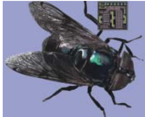
A common housefly dwarfs the 1.2 x 1.3-mm GMR sensor to be used in Starkey Labs' hearing aids.
