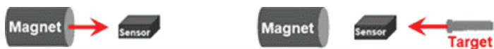
Two proximity sensing configurations -- magnet detection at left, and back-biased configuration at right, enable detection of either permanent magnets or ferromagnetic objects.
