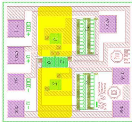
Fig. 2. Layout of Commercial GMR Multilayer Sensor
