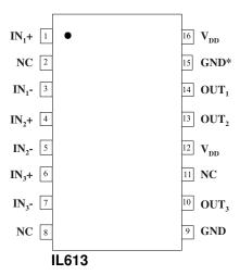
Note: Pins 12 and 16 must be connected externally.
