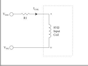
Figure 2. Limiting Resistor Calculation Equivalent Circuit
