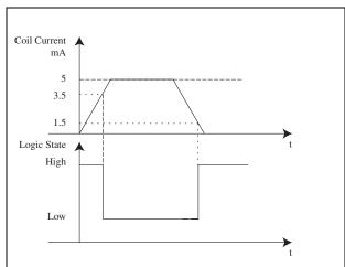
Figure 1. Typical IL600-Series Transfer Function
