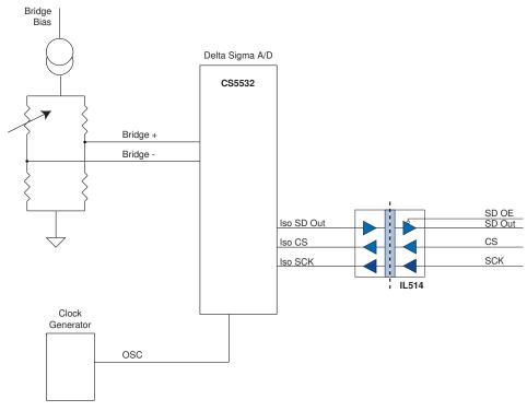
A delta-sigma A-D converter interfaced with the three-channel IL514. Multiple channels can easily be combined using the IL514's output enable function.
