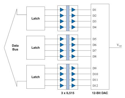
The IL515 four-channel isolator is ideally suited for parallel bus isolation. The circuit above uses three IL515s to isolate a 12-bit DAC.
