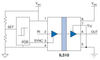
Fig. 1. Typical Power On Reset Circuit for IL510
