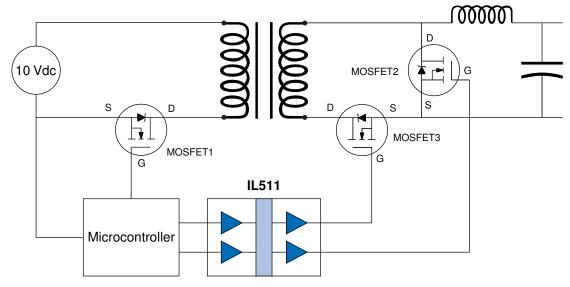
A typical primary-side controller uses the IL511 to drive the synchronous rectification signals from primary side to secondary side. IL511 pulsewidth distortion of 10 ns minimizes MOSFET dead time and maximizes efficiency. The ultra-small MSOP package minimizes board area.
