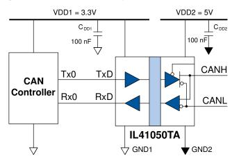
As Figure 3 shows, the IL41050TA can provide isolation and level shifting between a 5 volt CAN bus and a 3 volt microcontroller:
