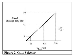
The boost capacitor in parallel with the current-limiting resistor boosts the instantaneous coil current at the signal transition. This ensures switching and reduces propagation delay and reduces pulse-width distortion.
