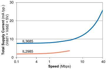
Figure 1. Supply current vs. speed.
