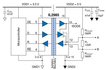
Figure 2. Typical connections.
