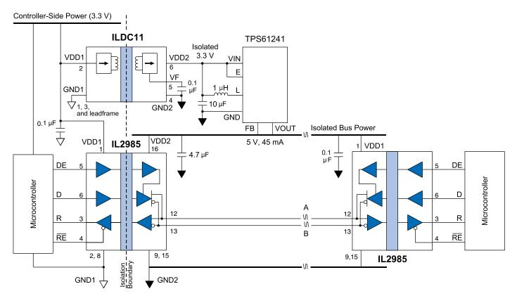
Figure 3. An RS-485 system with an ILDC11 isolated DC-DC convertor.
