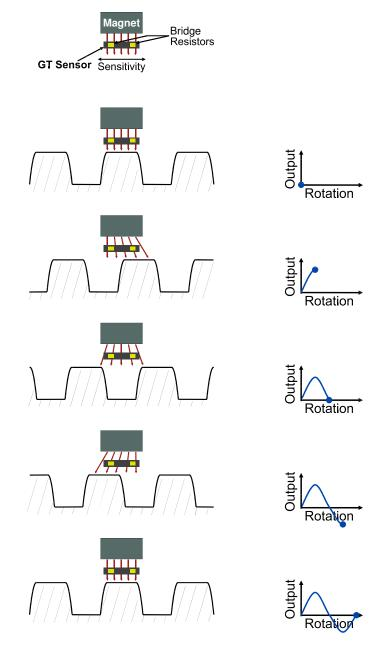
Figure 3. ABL00x output vs. gear rotation.
