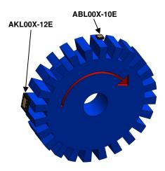
Figure 1. Sensor orientation.
