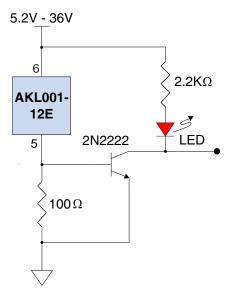
Figure 10. Simple three-wire interface.
