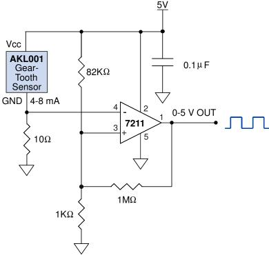
Figure 11. TTL output gear-tooth sensor.
