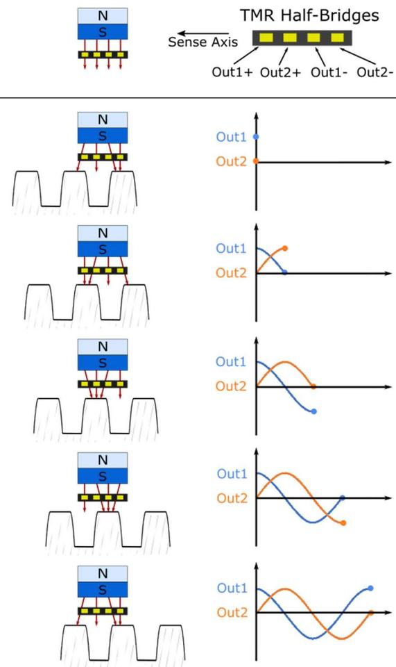
Cycling gear teeth create a sinusoidally varying field pattern from a fixed bias magnet. The ABT-Series sensors operate on this principle by detecting the tangential field gradient. For more information about AET-Series operation, read the datasheet and visit the sensor applications page:
