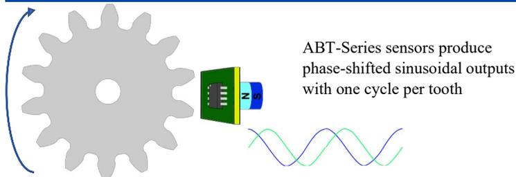
The ABT375 is an ultraprecise gear-tooth sensor that detects the periodic magnetic fields produced by magnetized gear teeth. The gear teeth are magnetized by fixing a back-biasing ceramic magnet symmetrically behind the sensor. The sensor is single-axis sensitive, and its spaced TMR elements are optimized for 1.5 mm pole pitch.
