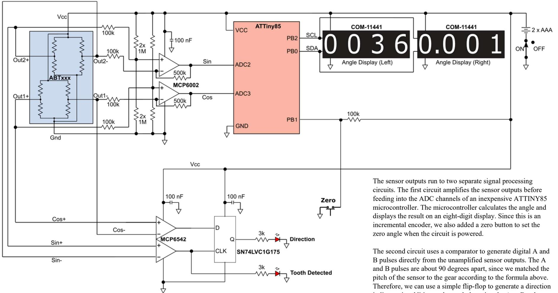
The sensor outputs run to two separate signal processing circuits. The first circuit amplifies the sensor outputs before feeding into the ADC channels of an inexpensive ATTINY85 microcontroller. The microcontroller calculates the angle and displays the result on an eight-digit display. Since this is an incremental encoder, we also added a zero button to set the zero angle when the circuit is powered.
