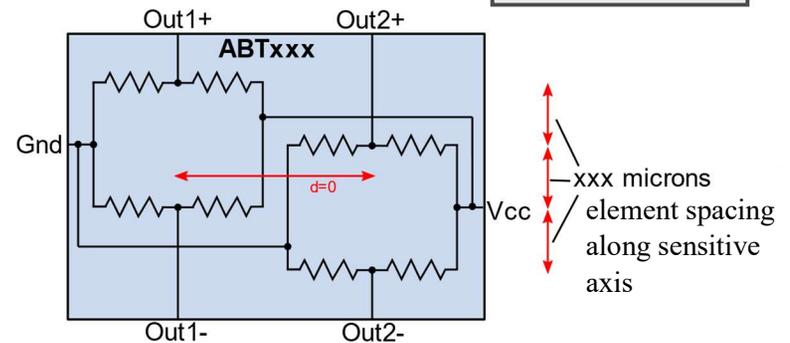
When a magnetic field gradient is swept along the sensor's sensitive axis, the four half-bridges produce identical, phase-shifted outputs corresponding to the pitch of the field gradient. In the case of a gear, the phase-shifted magnetic field is due to the gear-tooth pitch:
