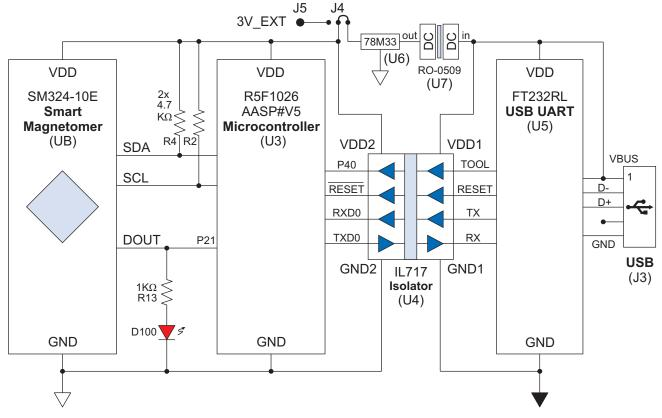
Figure 3. Simplified Board Schematic.
