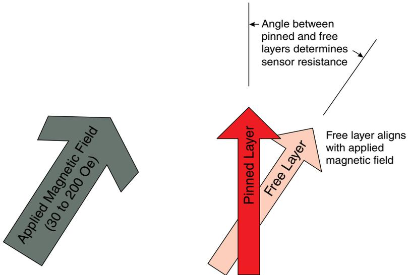
The sensor element free layers will align with the external field. As the applied field changes direction, the angle between the free layer and the pinned layer changes, changing the resistance of spintronic Tunneling Magnetoresistance (TMR) elements, which changes the device output voltages.
