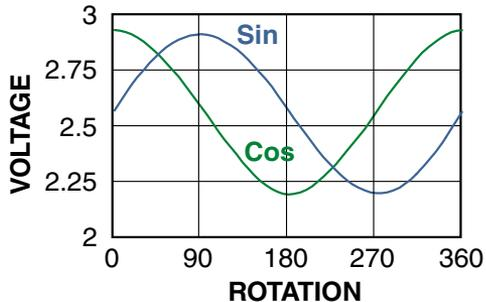
The output is insensitive to magnet spacing over a wide range. Signal is lost if the magnet is too far away; if the magnet is too close the outputs will be non-sinusoidal. A relatively large magnet-sensor airgap is possible with the magnet provided with the kit, although smaller magnets will require a smaller gap.
