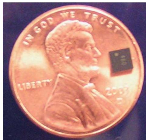
Figure 4. Photo of a spin valve rotation sensor packaged in a leadless TDFN6 format (on a penny background).
