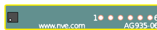
Figure 15. AG035-06 bare circuit board for TDFN6 sensors. 1.57" x 0.25" (40mm x 6 mm) (actual size)
