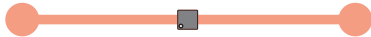
Figure 4a. 0.05" (1.3 mm) trace on top of PCB (2.8 Oe/amp; 0 to 3.5 A linear range).
