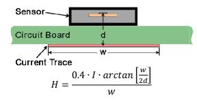
where the magnetic field H is in millitesla, the width of the trace w in mm, and d is in mm. The AG905-06 produces 0.023 mT/amp at the sensor, which corresponds to ±220 amps in the sensor's highly linear ±5 mT range.
