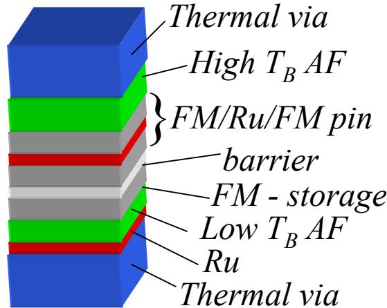
Offset field ( $H_{ex}$ ) drops to zero at high temperature ( $T_B$ )
