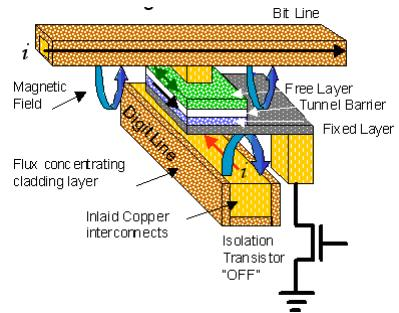
Control of the distribution of switching fields makes the SW-MRAM implementation difficult to manufacture and scale.
