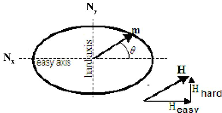
$$E = -\frac{1}{2}(N_y - N_x)M_s^2 V \sin^2 \theta - M_s(H_{\text{easy}} \cos \theta + H_{\text{hard}} \sin \theta)V$$
