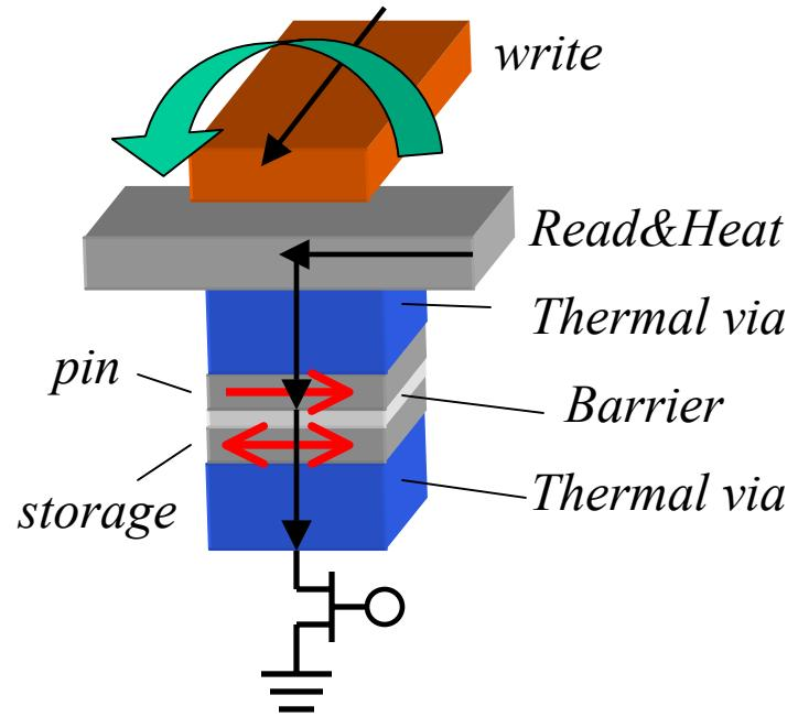
Goal: Design for high density → Heating current below 100  $\mu$ A at 100 nm bit size
