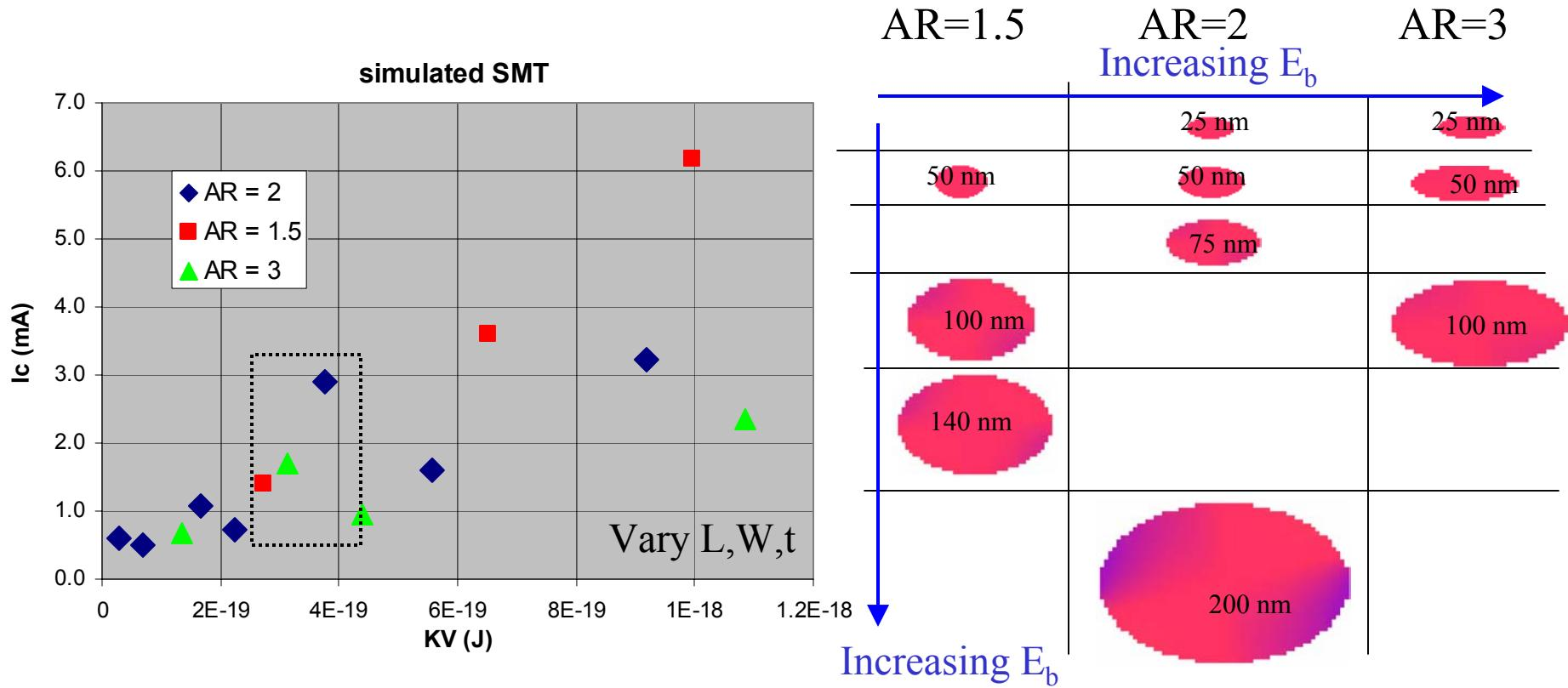
$E_b$  must remain high as bit size is scaled down – thickness must increase
