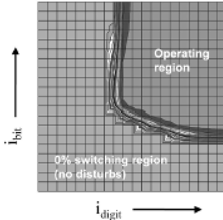
Thermal stability at small bit size still an issue → high write current
