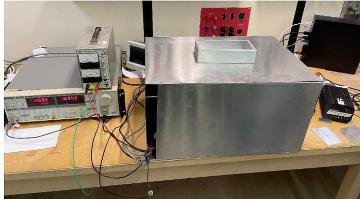
*Figure 9: Finalized testing design with faraday cage*
