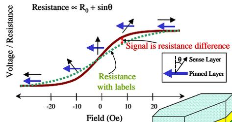
The green dashed curve represents the measured resistance when beads are present, and the solid curve is the initial resistance.
