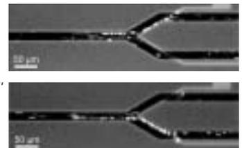
Photos of 2.8 micron Dynal beads (w / fluorescent dye) deflected left or right depending on + or - electrical current
