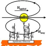
Detector sees  $H_{Total} = H_{applied} + H_{stray}$  along a designed sense-axis. In the example here, the stray field is opposite in direction to the applied field. The magnitude of the stray field is strongly dependent on the distance from the label. Labels can be easily detected within about 1 diameter, but the signal falls off as distance<sup>3</sup>.
