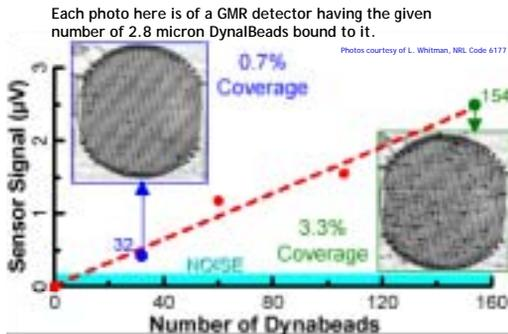
The measured sensor voltage is indicated by the vertical axis. Each sensor is about 200 µm in diameter. The beads show up as black spots. This detector has a linear response of signal vs. number of beads over about 2 to 3 logs.
