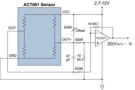
This op-amp circuit has a gain of 20 for full-scale at approximately the sensor's maximum output. The potentiometer provides a positive offset so negative currents still produce a positive output, and corrects the sensor's offset. The 500 k $\Omega$  input resistors are significantly higher than the sensor output impedance to avoid loading. The capacitor limits high-frequency noise. The low-cost, low bias current op amp allows large resistors to avoid loading the sensor bridge.
