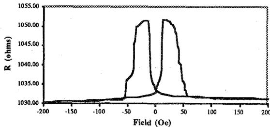
Fig. 2. R-H plot for a 10 $\mu\text{m}$ X100 $\mu\text{m}$  SDT device.
