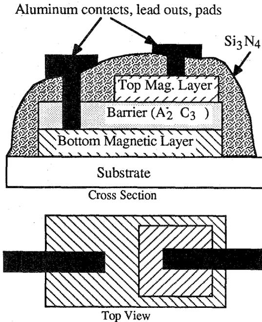
Fig. 1. Top view and cross section of a SDT device. The remaining top magnetic layer defines the active area of the device.
