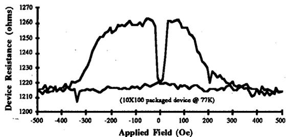
Fig. 5. R-H plot of a SDT device at 77 K. The hard layer saturation field has increased by a factor of 5 from the room temperature value. Base resistance has increased by 20%.
