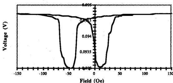
Fig. 6. SDT characteristic with a bias applied by an integrated bias strap. For the proper "set" of the hard layer, a bipolar response is obtained from bipolar fields.
