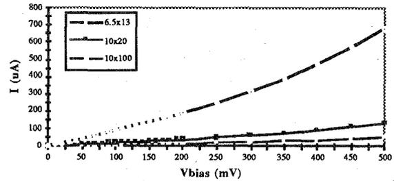
Fig. 3. Representative I-V curves for the three different SDT device types.
