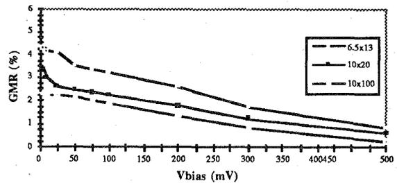
Fig. 4. GMR versus bias voltage for SDT devices. Based on this characteristic, these devices will be inherently low voltage, low power devices.
