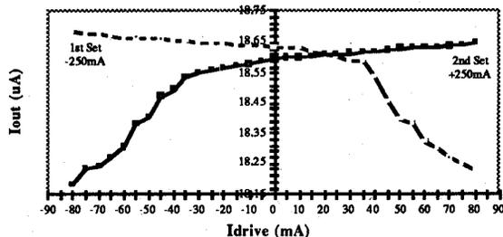
Fig. 7. "Read" traces of a SDT device following a write to a "0" state and to a "1" state.
