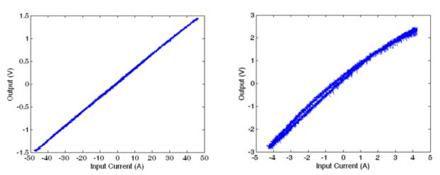
Figure 7. Linearity of the current sensor (a) with Helmholtz coil and; (b) without Helmholtz coil.
