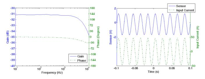
Figure 8. (a) Frequency response of the sensor; (b) waveform of the input current and the output of sensor at 50 Hz.
