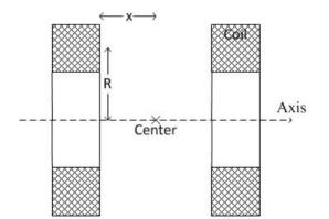
According to the Biot-Savart law, the magnetic field  $H_s$  generated by a single wire coil at the center point of the axis is:
