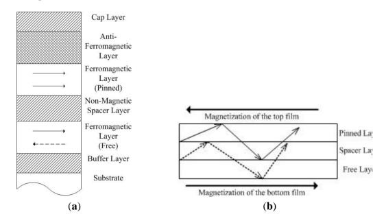
Figure 1(b) shows that the electron path is limited as the electrons scatter off the interface of the two ferromagnetic layers. It is because the magnetization direction changes the spin characteristics of the conducting electrons in magnetic materials. The current flows from left to right in the diagram. The electrons are referred to as "spin up electrons" in the top ferromagnetic layers, and electrons are
