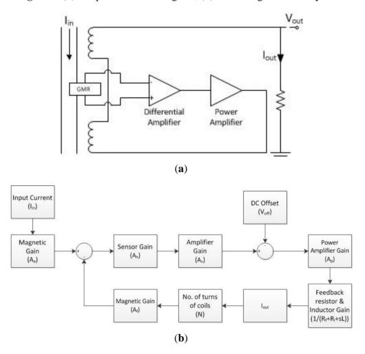
Figure 4. (a) Simplified circuit diagram; (b) block diagram of the system.
