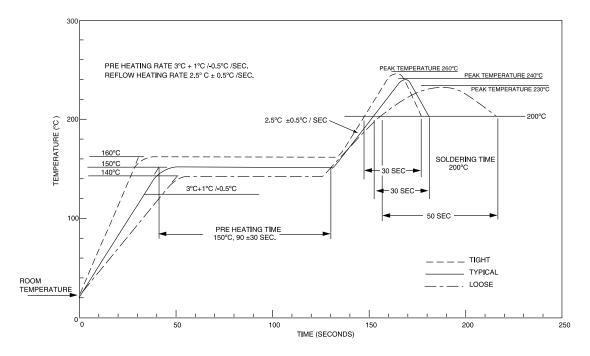
For leaded (Pb) parts, the peak temperature shown in this profile can be decreased to as low as 230°C. Exceeding 265°C at peak or the time at peak temperature shown in this profile can damage the parts. Specifically:
