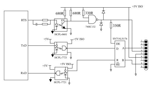
Fig. 1. Typical Profibus DP Node
