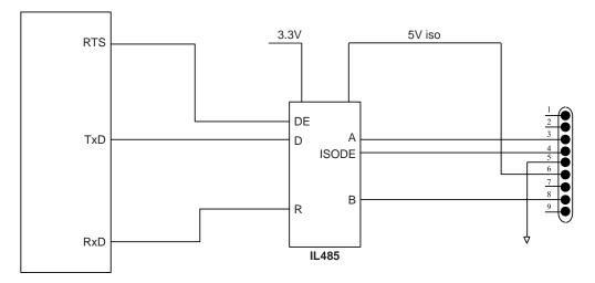
Fig. 2. Profibus DP Node using an IL485
