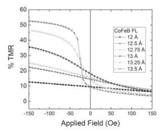
Evolution of the resistance versus applied magnetic field curves for MTJs with FLs ranging from 12 Å to 13.5 Å.
