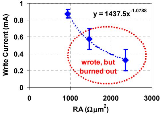
Figure 4. Write current for three different  $1 \mu\text{m} \times 1 \mu\text{m}$  magneto-thermal MRAM elements as a function of  $\langle RA \rangle$ . Writing current decreases as  $1/\langle RA \rangle$ , but large  $\langle RA \rangle$  causes the MTJ to breakdown before the blocking temperature of the storage layer can be reached
